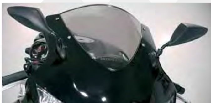
Attacco carena M.6 / Fairing connection M.6
